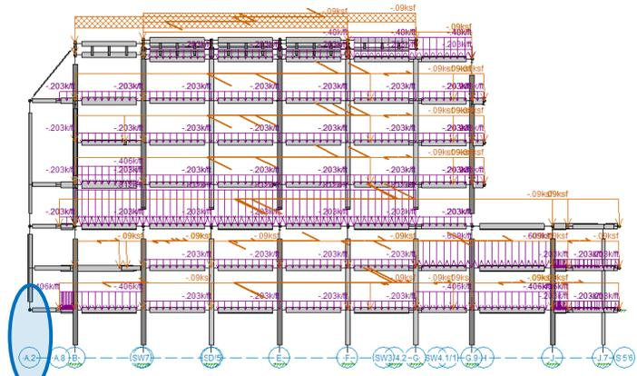
Figure 7.30 – Near Loading, including all dead loads. Column A.2-2.4, which is highlighted, was removed. Isometric View
